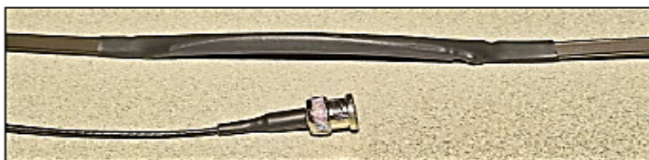
Figure 5 — The \lambda/4 UHF decoupling stub made of RG-174A, covered with heat shrink tubing. This is shown next to the BNC connector that goes to the transceiver.
