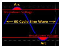
The resulting noise bursts repeat at 120 Hz, since the voltage breakdowns occur twice during each 60 Hz power cycle. The resulting radio frequency interference (RFI) may span the AM broadcast band to 30 MHz or beyond at various levels. In some cases the interference may only be detectable across portions of the HF spectrum.
